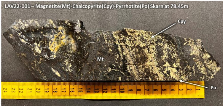
Figure 3: Photographs of HQ-sized core intervals representing upper Cu-bearing skarn, Mo mineralization in diamond drillholes LAV22-001 and LAV22-002 completed at the historic French Adit of the Laverdiere Project in 2022.
