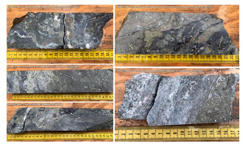
**Figure 2:** Photographs of representative 2022 HQ-sized core intervals from SLM22-003 and SLM22-004 of base metal sulphide (Chalcopyrite = Cpy; Galena = Gn; Sphalerite = Sph; Pyrrhotite = Po; Pyrite = Py) occurrences at the Jackie Target, Silver Lime Project.
