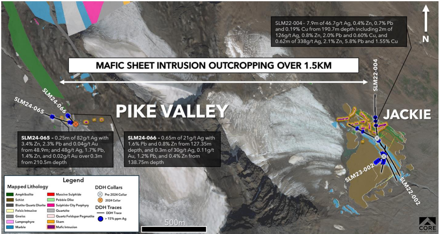
Figure 3: Plan view map of the Pike Valley and Jackie Targets illustrating drill core assay highlights for 2024 and 2022 in both areas related to a newly identified mafic sheet intrusion that host's widespread epithermal base metal veins.
